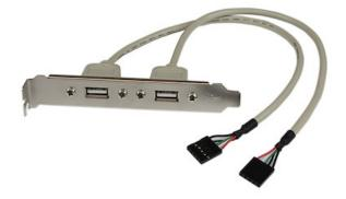
The USBPLATE 2 Port USB A Slot Plate converts the USB pins from most AT style Pentium (and newer) motherboards to 2 standard USB A-Style ports. The plate can be mounted on the rear panel of a computer case, adding two USB A female ports for simple connection to USB peripheral devices.
